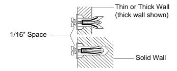
Figure 6 - Tightening Anchors
